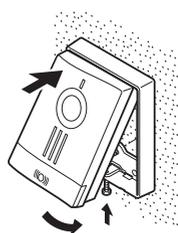
Insert the top section of the video door station into the mounting frame and push in the bottom section. Tighten the locking screw on the bottom to secure the video door station.
