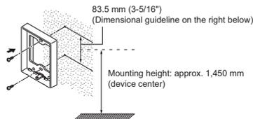
Secure the stand using the two included screws or wooden screws.
