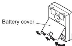
Loosen the two screws and remove the battery cover.
