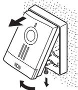
Loosen the locking screw of the bottom section, pull out the bottom section of the video door station first and pull out the top section.
