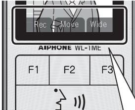
The functions displayed on the screen can be manipulated by the function button just below.
