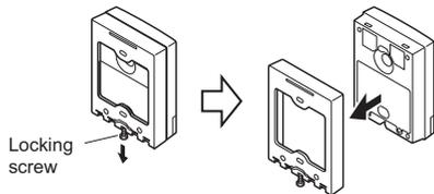
Loosen the locking screw on the bottom and remove the frame.
